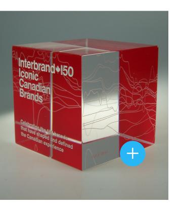
The back wall of the cube, the central part of the design, was printed three times. The first print laid down the red base of the design, the second created the white lines of the 'topography' and the third pass – an overlay of red – made it come to life.
